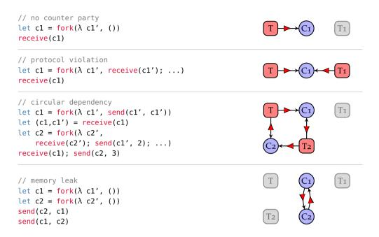
Figure 4: Examples of configurations that are deadlocked or have leaked.
