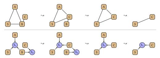
Figure 16: Steps in three buyer protocol. Top: physical communication paths; bottom: logical connectivity.
