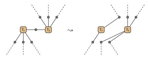
On the left,  $T_1$  and  $T_2$  each own 3 barriers, and they are also connected by a barrier. On the right, after the synchronization has taken place, the barrier between them has disappeared. Two of the barriers of  $T_1$  were transferred to  $T_2$ , and one of the barriers of  $T_2$  was transferred to  $T_1$ . Once again, if the graph on the left was acyclic, then the graph on the right will still be acyclic.<sup>6</sup>
